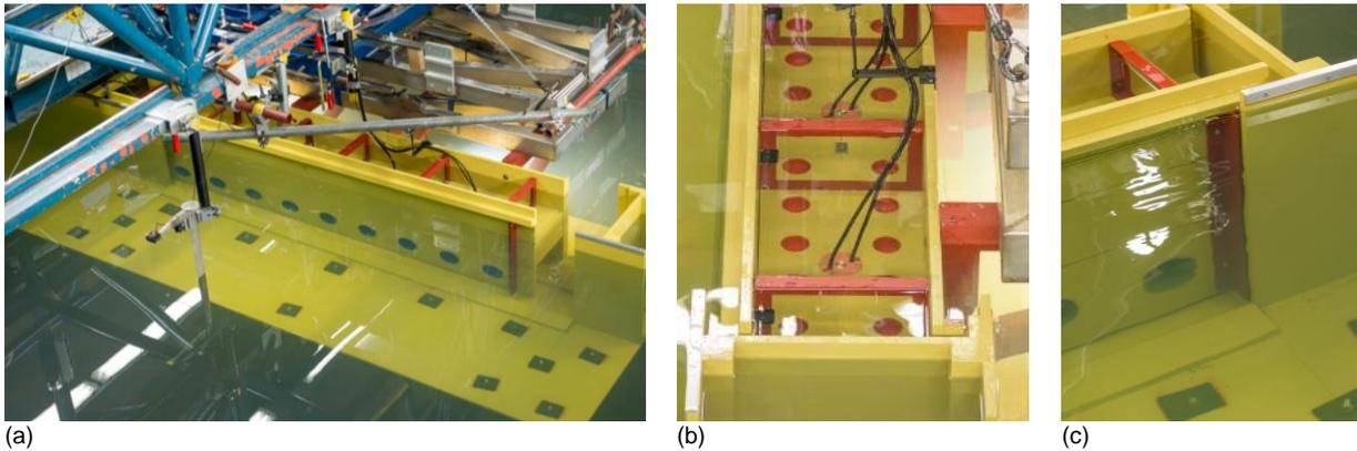
**Figure 7: (a) Overall view of the test setup. (b) Side top view of the scale model in the basin; the plastic caps to close off the vertical tubes are visible; pressure sensors were installed on the top and bottom of the ballast tank as well to validate the force measurements. (c) Side plating to close of the gate recesses.**
