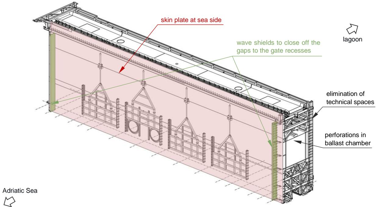
**Figure 11: Redesigned sea side lock gate: design improvements.**
