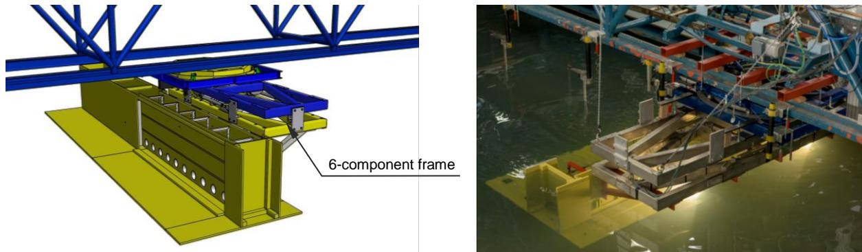
**Figure 8: 3D rendering of the six component frame attached to the scale model & picture of the setup in the test basin.**
