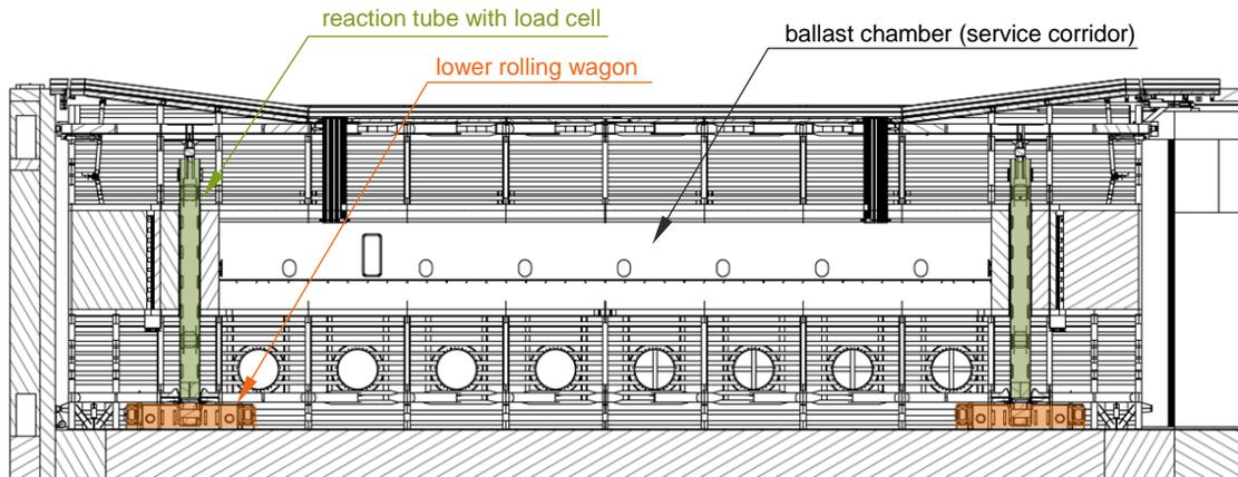
**Figure 14: Redesigned sea side lock gate: cross section.**
