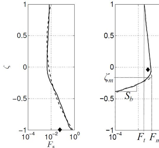
**Figure 10: Vertical profile of  $F_s$  for two types of plumes. CFD results in full lines, parameterisations in dashed lines, preliminary plume centerline position in black diamond. Near-bed density current type with Chebychev parameterization (left panel). Right panel shows the 'detached' plume type with step-wise parameterisation (dashed line), defined by (co-) ordinates  $\zeta_m$ ,  $F_t$  and  $F_m$  and the slope  $S_b$ .**
