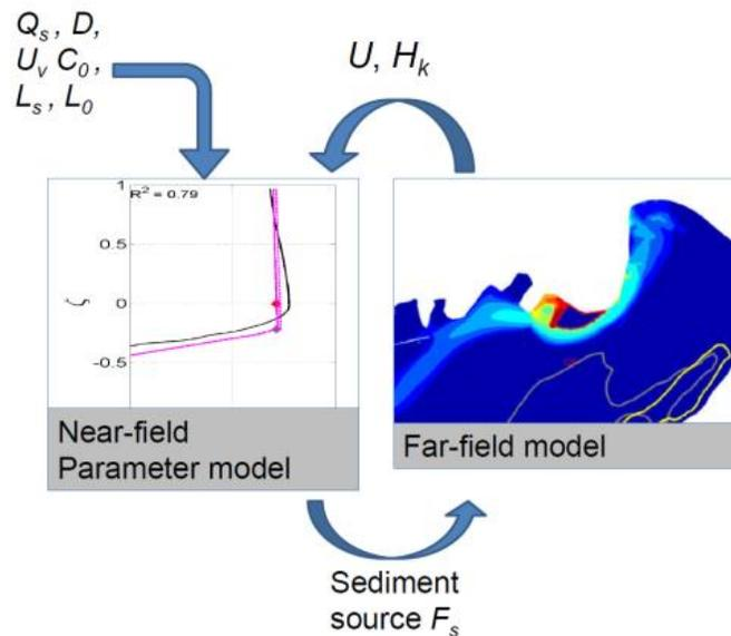
Figure 12. Schematic representation of the online coupling between near-field parameter model and far-field hydrodynamics/plume dispersion in TELEMAC.
