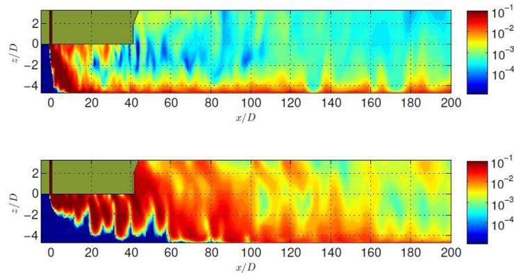
Figure 6. CFD results (relative concentration  $c/C_0$ ) with low dredging speed (top panel) and with high dredging speed and/or head current (lower panel).
