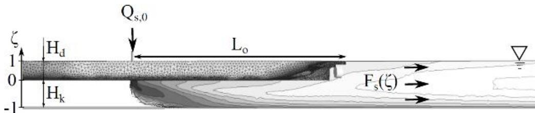
Figure 8. Definition sketch of the parameter model and variables used therein.
