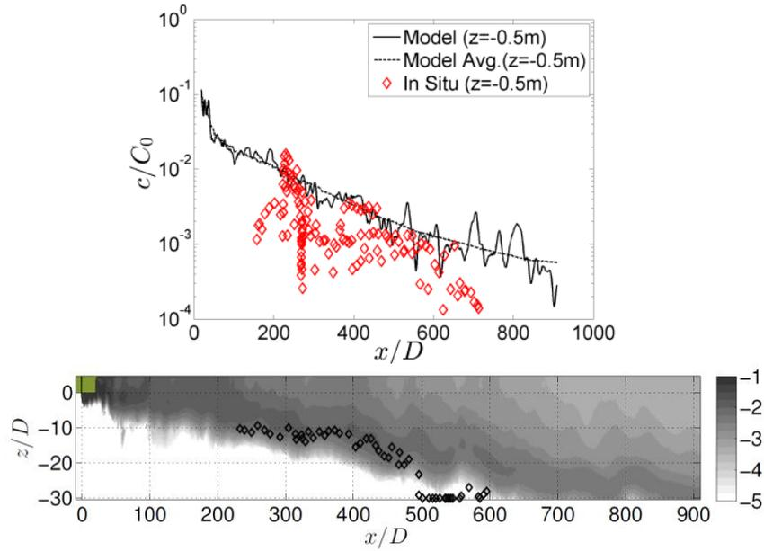
Figure 4. Upper panel: range of observed sediment concentration  $c/C_0$  (red markers) compared to the centerline (maximum)  $c/C_0$  values from the CFD model. Lower panel: Vertical slice of CFD sediment concentration  $\log(c/C_0)$  (along the ship axis, in grayscale), compared to the lower edge of the plume as observed in the field (black diamonds).
