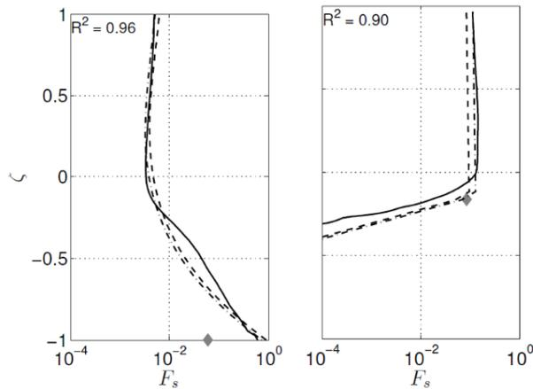
Figure 11. Two validation cases for the parameter model. Full lines represent vertical profiles of sediment flux from the CFD model, dashed lines are the results of the parameter model (before and after a corrector step ensuring the sediment flux continuity is respected).
