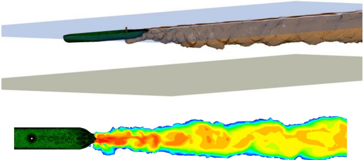
Figure 5. Examples of the turbulent sediment plumes computed using the CFD model. The isosurface connecting the locations at which  $c/C_0 = 10^{-4}$  is shown in the top panel. The lower panel gives a top view of the computed sediment concentration at the surface.
