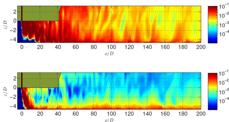
Figure 7. CFD results (relative concentration  $c/C_0$ ) with low  $C_0$  (10 g/l; top panel) and with high  $C_0$  (150 g/l; lower panel).
