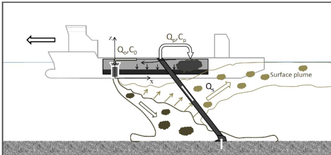
**Figure 1. Sketch of a Trailer Suction Hopper Dredger, pumping a water-sediment mixture (mass concentration  $C_p$ ) towards the hopper, at volume discharge  $Q_p$ . The sediment mixture settles while flowing towards the overflow, where a lighter mixture with sediment concentration  $C_0$  is released, with discharge  $Q_0$ .**
