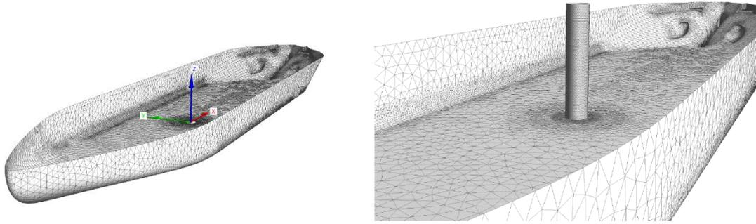
**Figure 3. Details of the surface mesh at the TSHD hull and overflow shaft walls.**
