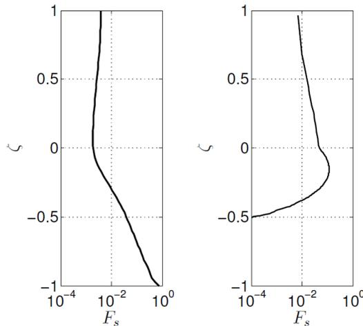
**Figure 9: Vertical profile of  $F_s$  for two types of plumes: Near-bed density current type (left panel) and the seabed-detached plume (right panel).**
