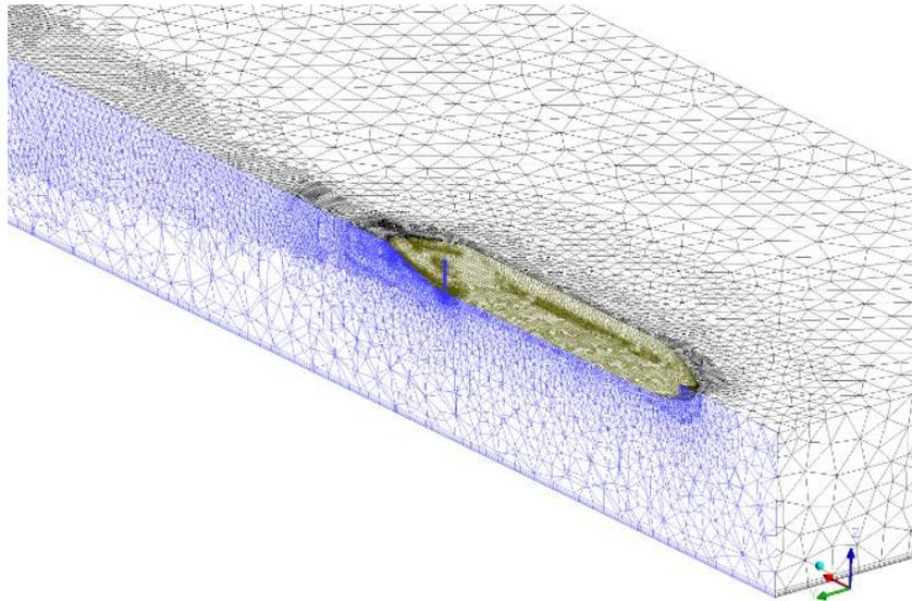
**Figure 2. Example of a model grid, tailored to a specific plume case for computational efficiency. Grid is sliced along the ship axis. Ship hull grid in brown, water surface grid in black, subsurface grid along slice in blue.**
