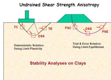
Fig. 8. Applicability of strength modes to foundation and embankment stability
