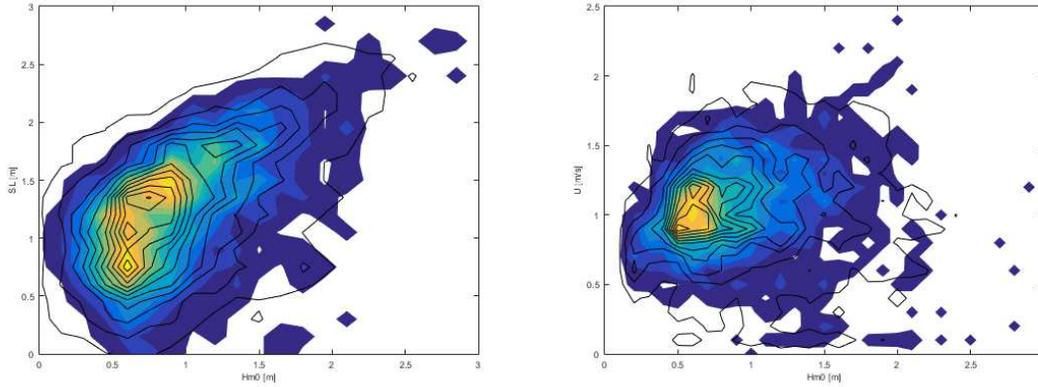
**Figure 12 – Empirical bivariate distribution of significant wave height and total sea level (left) and significant wave height and current speed (right). Original data in color and simulated data (one useful life) in black continuous lines.**
