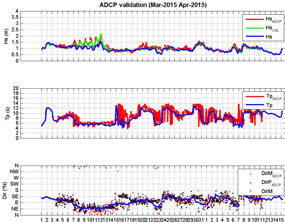
**Figure 3: Example of time series validation of the significant wave height (Hs), peak period (Tp), and mean wave direction (DirM) of the original Operational System (blue), the Calibrated Operational System (green) and ADCP measurements in the Port of Açú (red), from March 3, 2015 to April 11, 2015.**
