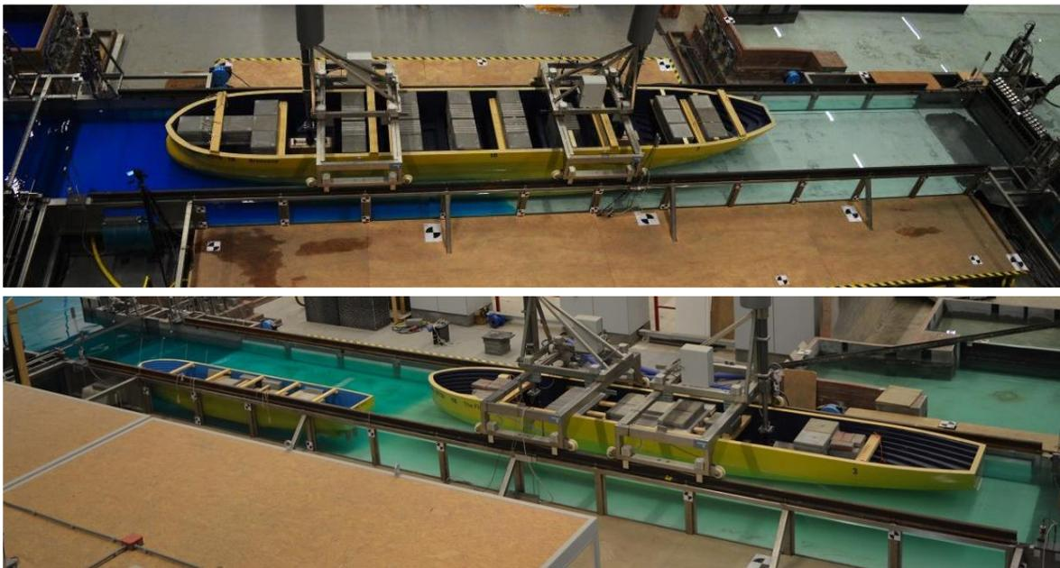
**Figure 3: The vessels used in the scale model study of the new lock of IJmuiden during a lock-exchange, with *Breesaap* (above) and *The Flying Dutchman* (below, on the right). In the lower panel also a smaller vessel has been moored in the lock to investigate the effect of multiple vessels in the lock chamber at the same time.**
