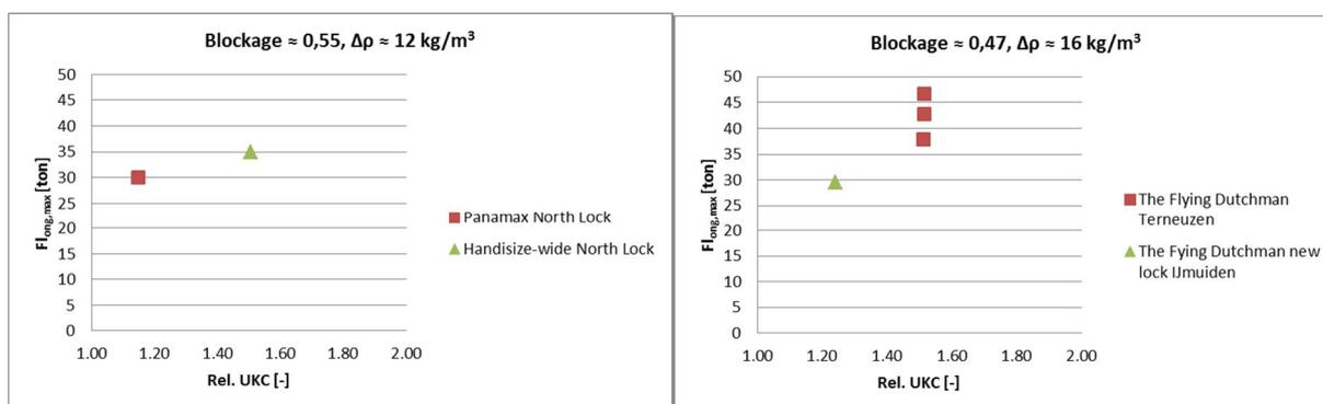
**Figure 8: Illustration of the influence of the relative under keel clearance (UKC) on the maximum longitudinal force for test with similar density difference and blockage. Left panel: outer head tests in the North Lock of IJmuiden for two different vessels (field measurements). Right panel: inner head tests for two different locks with *The Flying Dutchman* (scale model measurements).**
