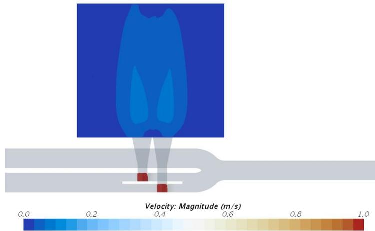
**Figure 10: Top view of velocity field above the bottom grid by emptying**
