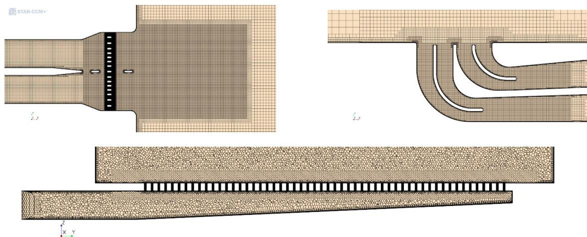
**Figure 6: Detailed views of the areas of local mesh refinement for the models of the outlet at the inner harbor (top left), the outlet at the outer harbor (top right), and, the chamber below the bottom grid and the bottom grid (below)**
