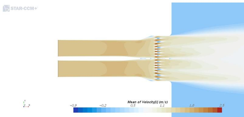
**Figure 7: Top view of mean velocity field for the outflow at the inner harbor when emptying the lock**
