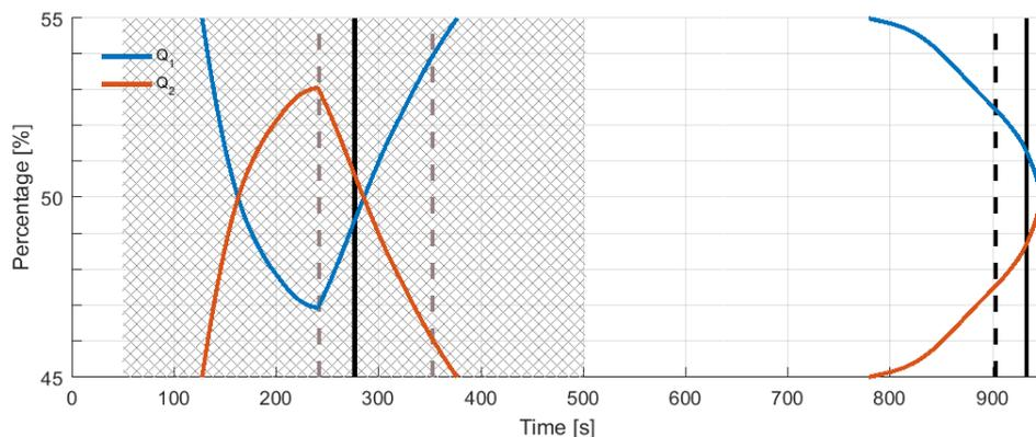
**Figure 17: Discharge through different bottom grids during levelling for Sim 6 as a percentage of the total discharge. The vertical solid black line is the moment of maximum total discharge. The shaded area is the period  $\pm 25\%$  of the total levelling time around the moment of maximum discharge**
