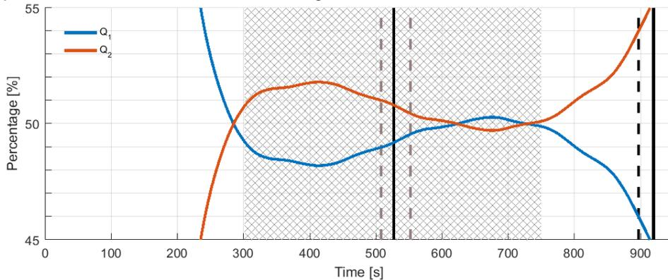
**Figure 16: Discharge through different bottom grids during levelling for Sim 5 as a percentage. The vertical solid black line is the moment of maximum total discharge. The shaded area is the period  $\pm 25\%$  of the total levelling time around the moment of maximum discharge**
