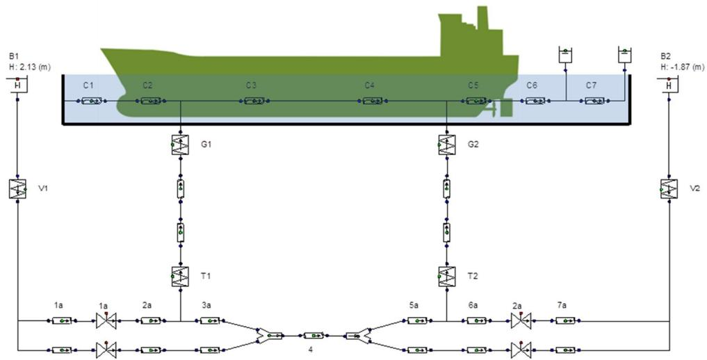
**Figure 11: Schematic view of the WANDA model**
