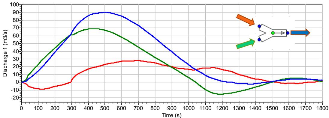
**Figure 14: Discharge through different culvert elements adjacent to the Y-junction during levelling for Sim 1. The definitions of the positive sense of discharges (the red, green and blue lines) is depicted with the corresponding coloured arrows around the Y-junction in the graph**
