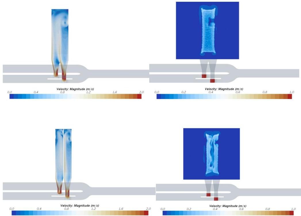
**Figure 9: Top view of velocity field for the bottom grids, left in the chamber below the grids and right in the lock chamber above the grids. The top two figures are for a bottom grid with a single spacechamber and the bottom figures are for a bottom grid with two separate spaces under the gridlower chambers.**
