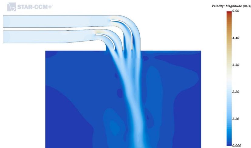
**Figure 8: Top view of velocity field for the outflow at the outer harbor when emptying the lock**
