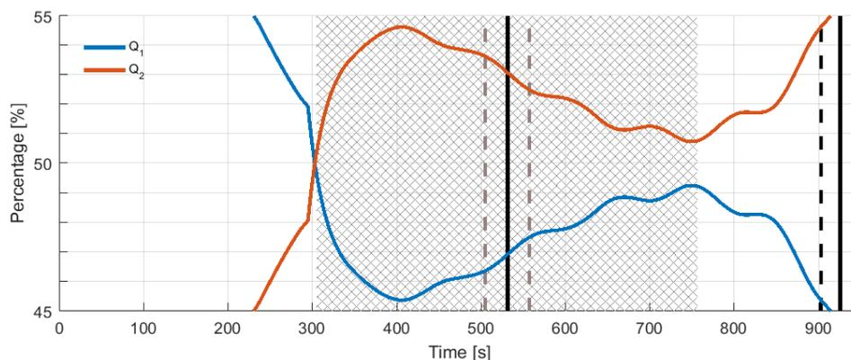
**Figure 15: Discharge through different bottom grids during levelling for Sim 1 as a percentage of the total discharge. The vertical solid black line is the moment of maximum total discharge. The shaded area is the period  $\pm 25\%$  of the total levelling time around the moment of maximum discharge**
