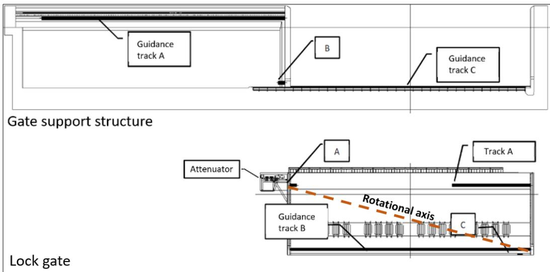
**Figure 13: Gate schematization and location of supports**
