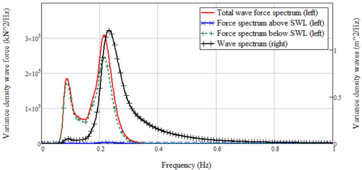
Figure 11: Longitudinal wave force variance density on gate
