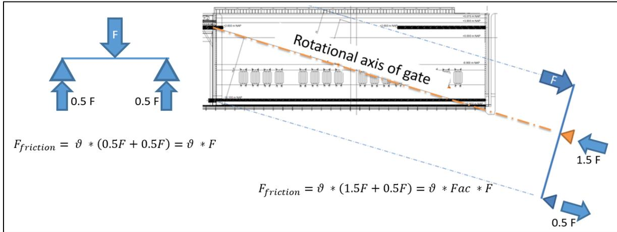
**Figure 12: Mechanical behavior of a simple supported beam and the lock gate**
