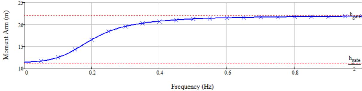
**Figure 14: Moment arm as function of wave frequency**
