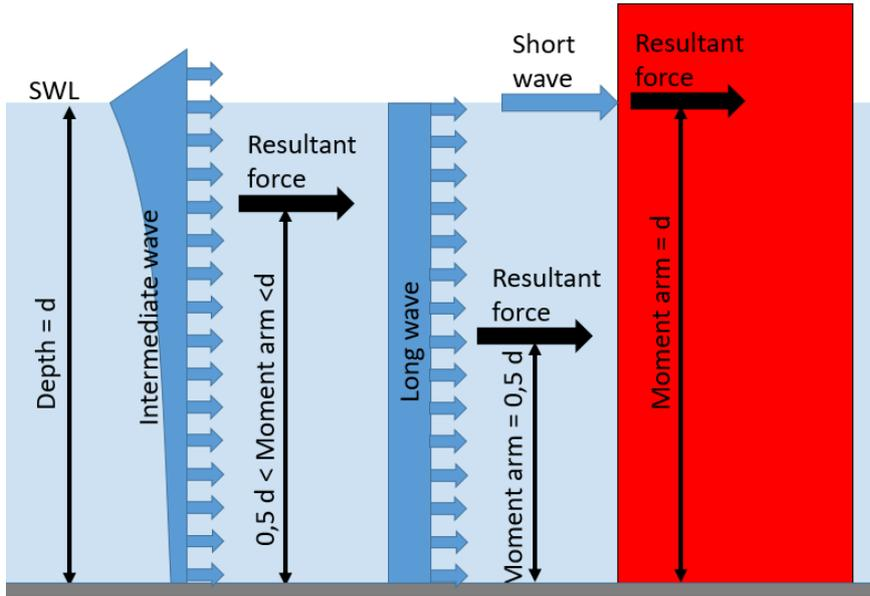
Figure 4: Wave forces acting on lock gate
