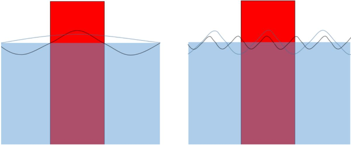
**Figure 9: Waves at the end of the gate. Left: gate loaded by long waves, right: gate loaded by short waves.**
