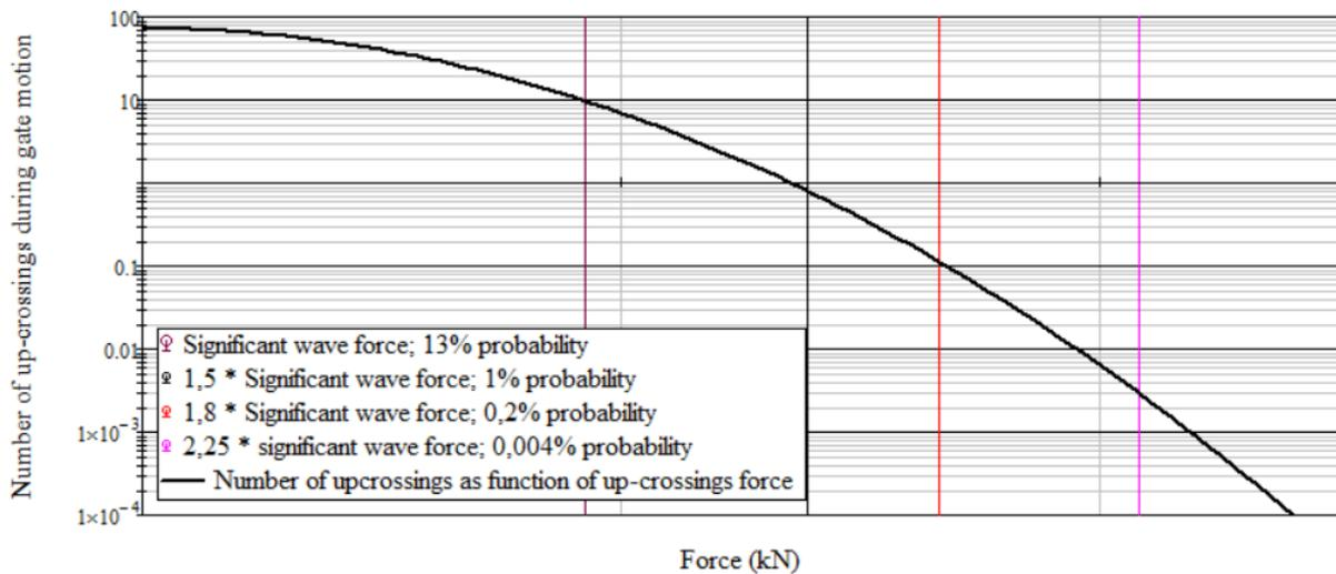
Figure 20: Number of up-crossings through level  $\eta$  during gate motion
