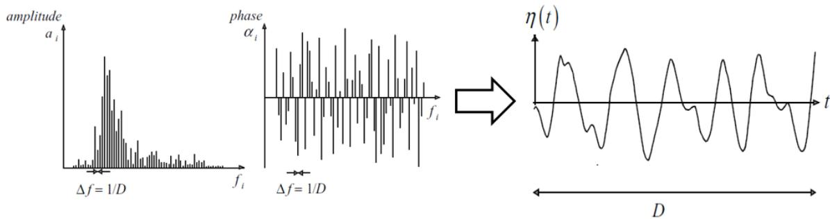
**Figure 21: Generation of a time series (Based on (Holthuijsen, 2007))**
