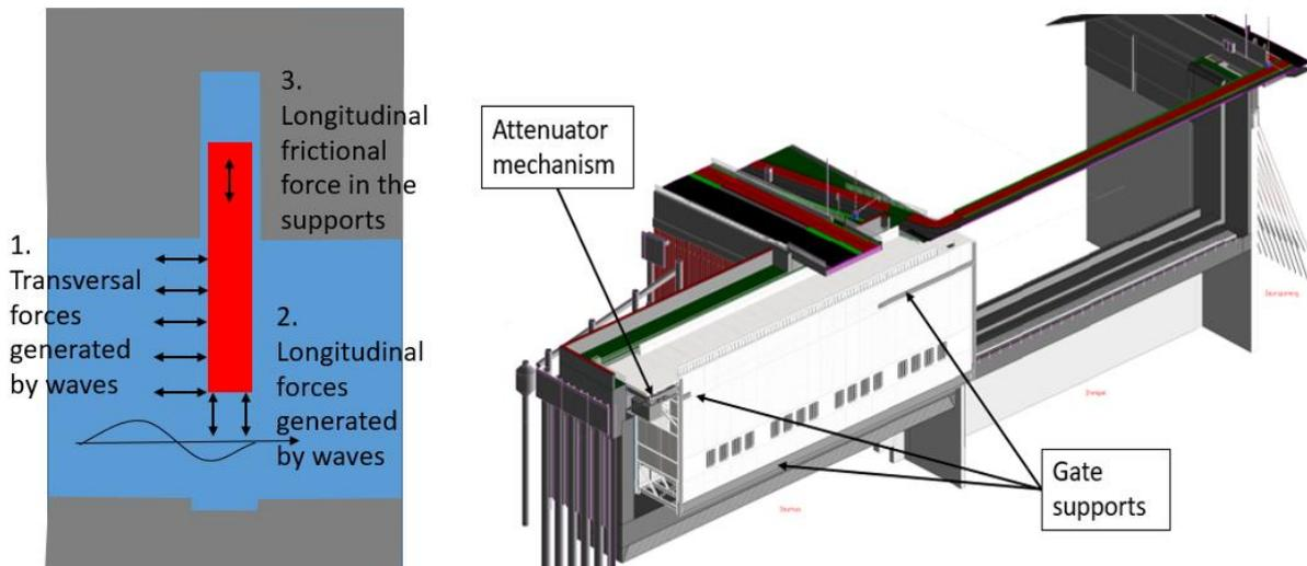
Figure 2: Overview of wave forces on the gate
