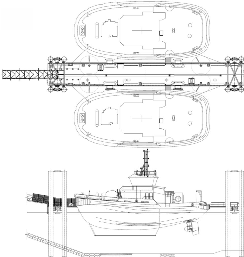
**Figure 9: Operational mooring arrangement**
