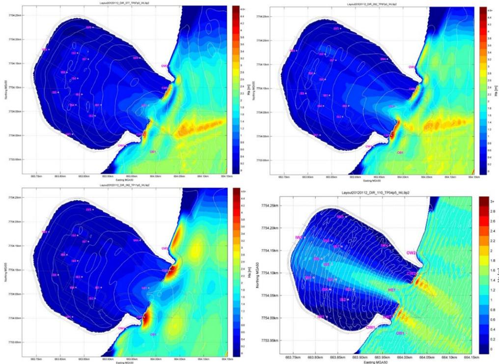
**Figure 3: Example wave penetration modelling results for a 500 years ARI storm tide of 9.2m. Model boundary waves as follows: (top left)  $T_p = 7s$ ,  $h_{sig} = 2m$ ,  $dir = 77^\circ TN$ , (top right)  $T_p = 7s$ ,  $h_{sig} = 2m$ ,  $dir = 92^\circ TN$ , (btm left)  $T_p = 11.5s$ ,  $h_{sig} = 2m$ ,  $dir = 92^\circ TN$ , (btm right)  $T_p = 4.5s$ ,  $h_{sig} = 1.4m$ ,  $dir = 110^\circ TN$**
