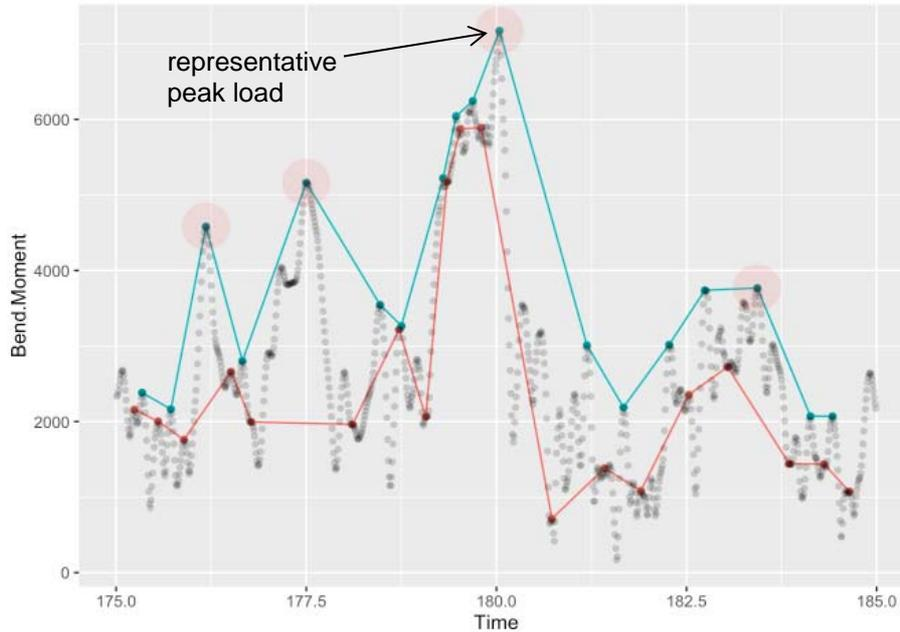
**Figure 5: Cyclic load assessment – finding representative peak pile loads showing raw data (black translucent dots), and the result of three passes of recursive local maxima finding (large red translucent dots). The blue line indicates local maxima included in the second and used for the final pass and the red line represents local maxima which were reclassified as local minima in the second pass.**
