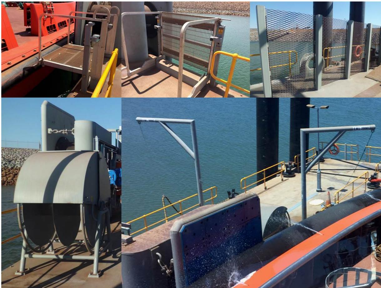
**Figure 8: Operability features (clockwise from top left): access brow lowered, access brow raised, snapback guards, mooring line hangers, cyclone mooring line reels**
