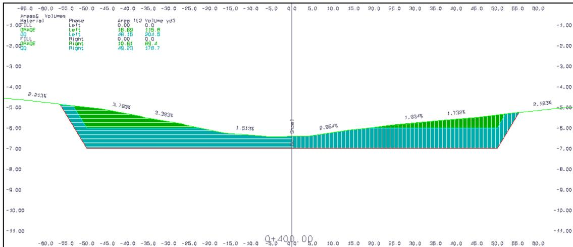
**Figure 1 – Typical cross section of data and design template during average end area calculations showing grade and overdepth regions**
