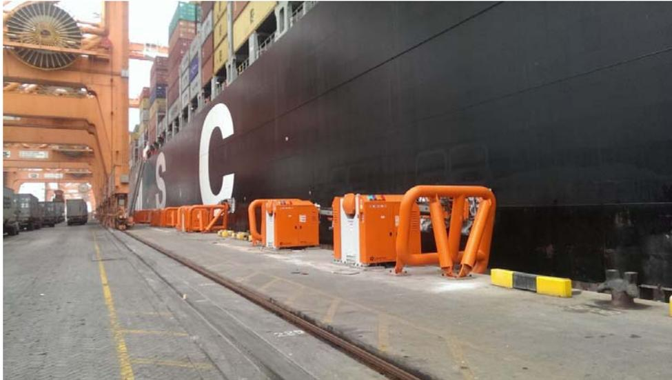
Cavotec MoorMaster™ MM400E<sup>15</sup> system installed in the Port of Salah
