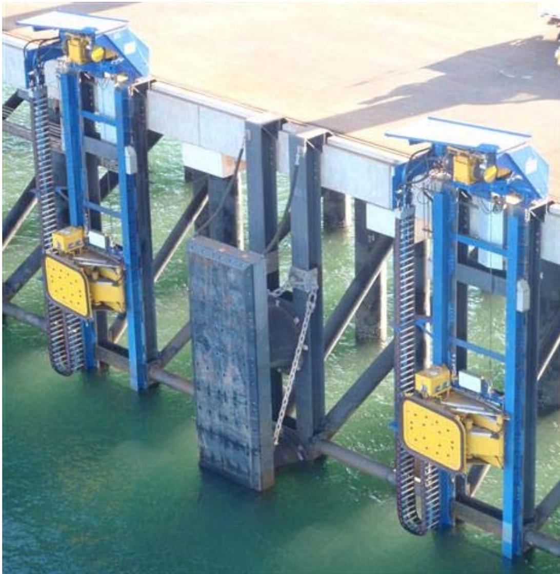
**Cavotec MoorMaster™ MM200C<sup>17</sup> system installed in Port Hedland**
