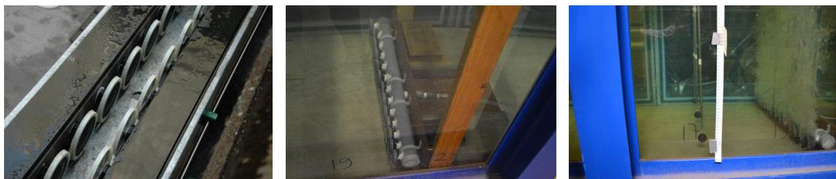
**Figure 7: Overview of scale model set-up by Van der Ven and Wieleman (2017): (a) bubble caps as built in the Kramer recreational lock; (b) caps used for the scale model of the bubble screen; (c) overview of the EMS instruments and bubble screen during a test condition**
