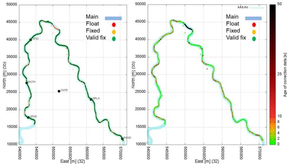
**Figure 6: data analysis (fix solution and data age) for AIS and GSM at Main test bed, Naab 10/2017**
