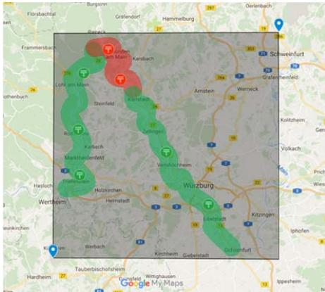
**Figure 4: Test bed Main River with additional AIS land sites transmitting on new VDES frequency channels (green) and area for GSM connection (red); Dark grey, regional area for frequency channels 2025 and 2026**
