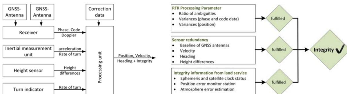
**Figure 3: On board processing with RTK algorithm and additional sensors (left). 3-stage integrity concept (right)**
