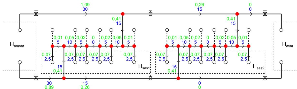
**Figure 4: Lock of Havré. Simplified estimation of head losses (in green) and discharges (in blue). Dashed lines in the culvert system are symmetrical parts. White nodes are connected with boundary levels; red nodes are internal junctions.**
