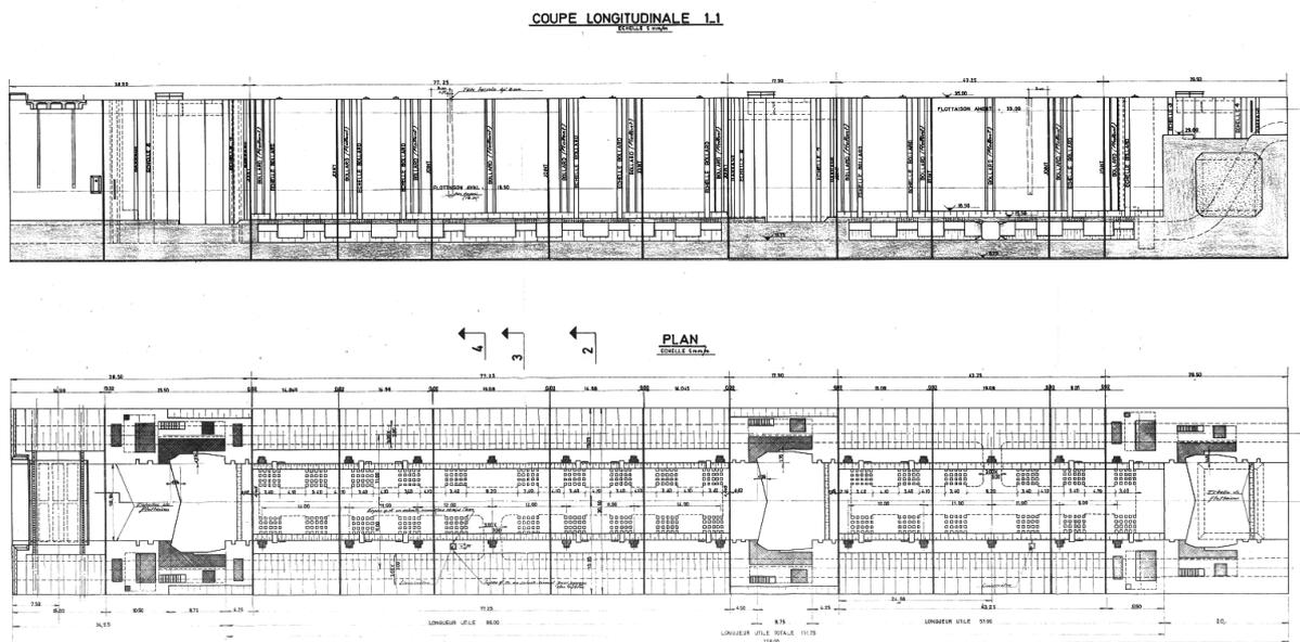
**Figure 11: Lock of Pommeroeul. Elevation and plan.**
