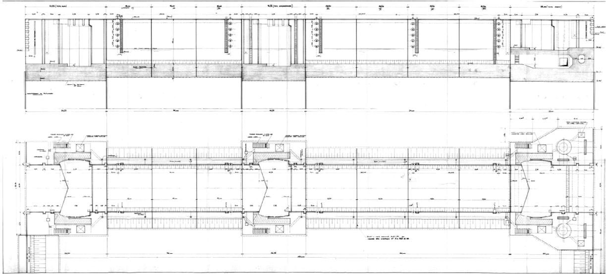
Figure 14: Lock of Hensies. Elevation and plan.
