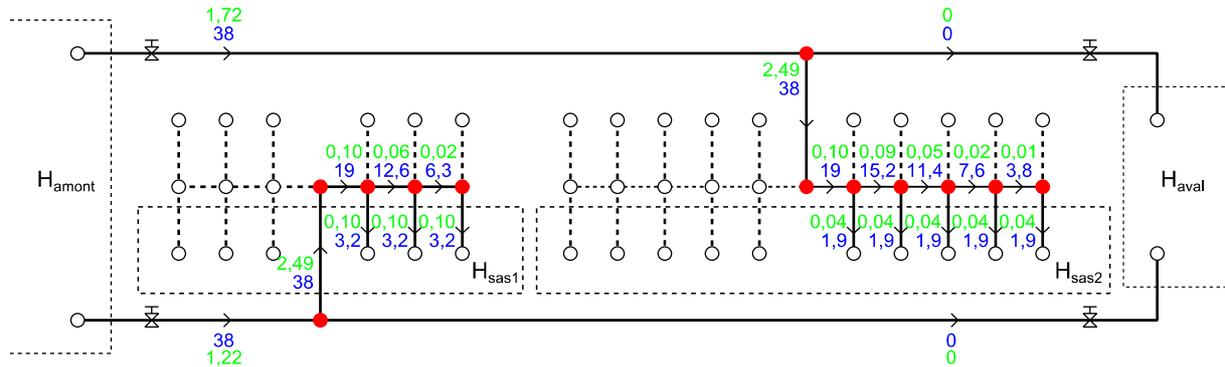
**Figure 12: Lock of Pommeroeul. Simplified estimation of head losses (in green) and discharges (in blue). Dashed lines in the culvert system are symmetrical parts. White nodes are connected with boundary levels; red nodes are internal junctions.**
