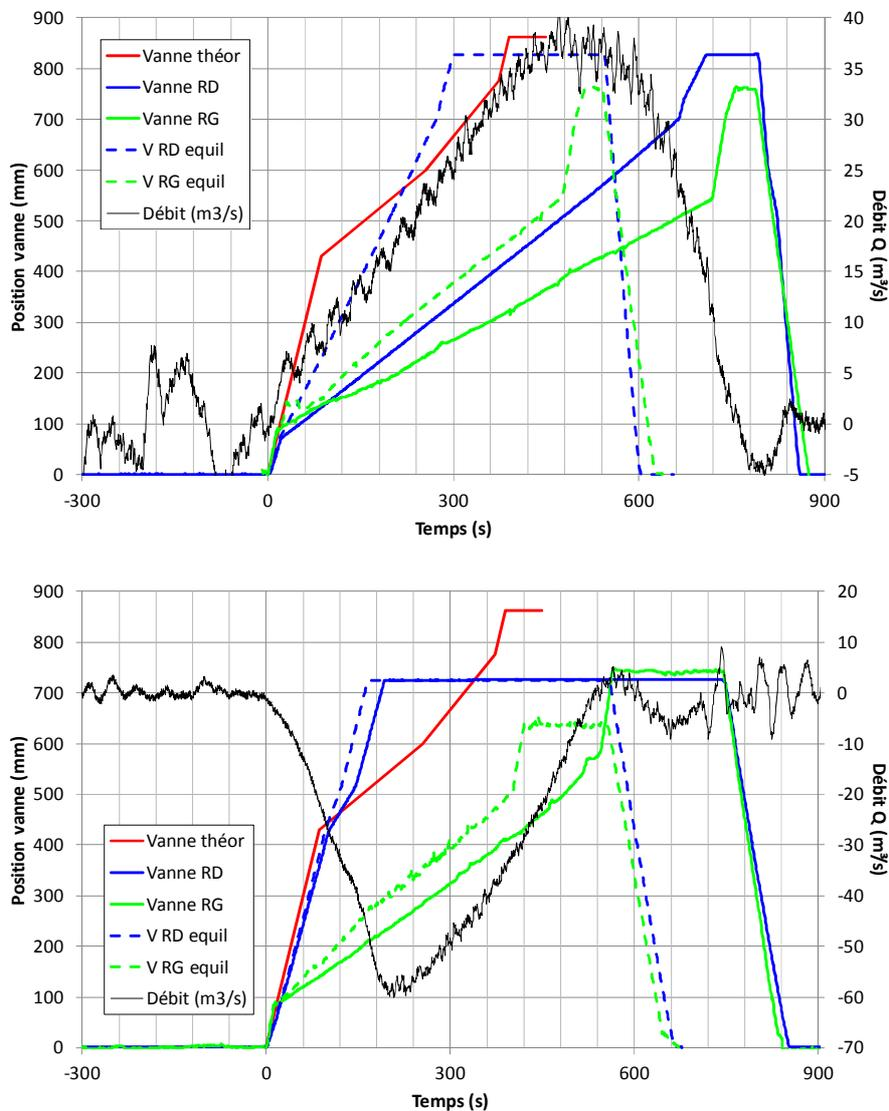
Figure 3: Lock of Havré. (a) Filling; and (b) emptying. Measured hydrogramme in black. Valve opening schedule (given as hydraulic jack position): theoretical curve (red), measured for right (RD-blue) and left (RG-green) valves. Plain curve is during levelling, while dashed curve is measured at equilibrium with no head on the valve.
