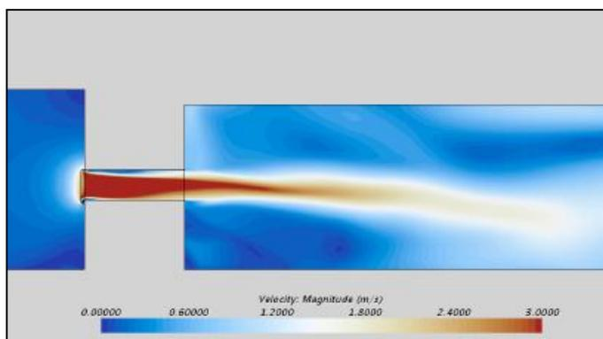
Figure 4: CFD Simulation, Flow Through Gate Ducts, Valve Fully Open,  $\Delta\rho = 20 \text{ kg/m}^3$
