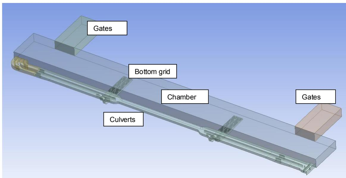
Figure 13: 3D CAD Rendering of Culvert System
