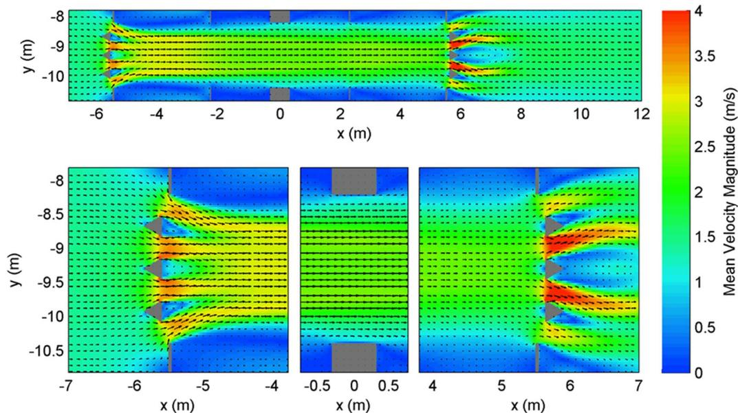
**Figure 10: Horizontal Cross-section of Duct; Flow Pattern: Water Flows to the Right**
