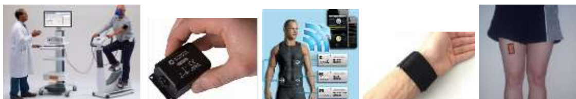
Figure 2: Examples of wearables and other sensors designed for measuring physical activity. From left to right: respiratory gas analysis, inertial measurement unit (IMU), smart sensor shirt, fitness bracelet and upper leg motion sensor.
