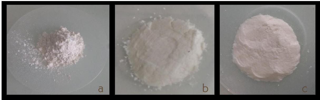
Photography of powder C, before sweat addition (a), during the mix with sweat (b), at sweat saturation (c)
