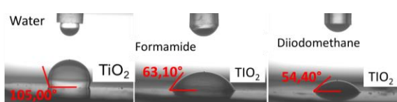
Figure 1: a) \text{TiO}_2 and b) Bentonite contact angle formed with water, formamide, and diiodomethane, the 3 reference solvents for the measure of the surface energy
