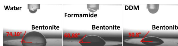
Figure 1: a) \text{TiO}_2 and b) Bentonite contact angle formed with water, formamide, and diiodomethane, the 3 reference solvents for the measure of the surface energy
