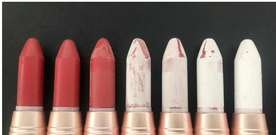
Figure 1 : Blooming phenomena on lipstick surface. Synthetic wax concentration from left to right in particular order : 0%; 0,5%; 1%; 3%; 5%; 7,5%; 11% (w/w).
