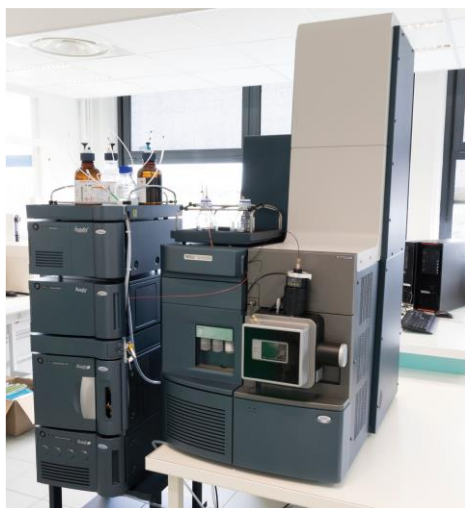
Figure 2. Picture of the LC-MS/MS system, a WATERS Xevo G2-XS Qtof coupled to an UPLC system WATERS ACQUITY UPLC I-Class used in this study.
