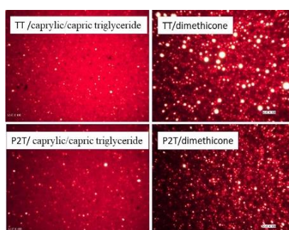
Figure 3B. digital microscopic images of w/o emulsions using TT and P2T treated iron oxide and caprylic/capric triglyceride and Dimethicone oil, respectively.
