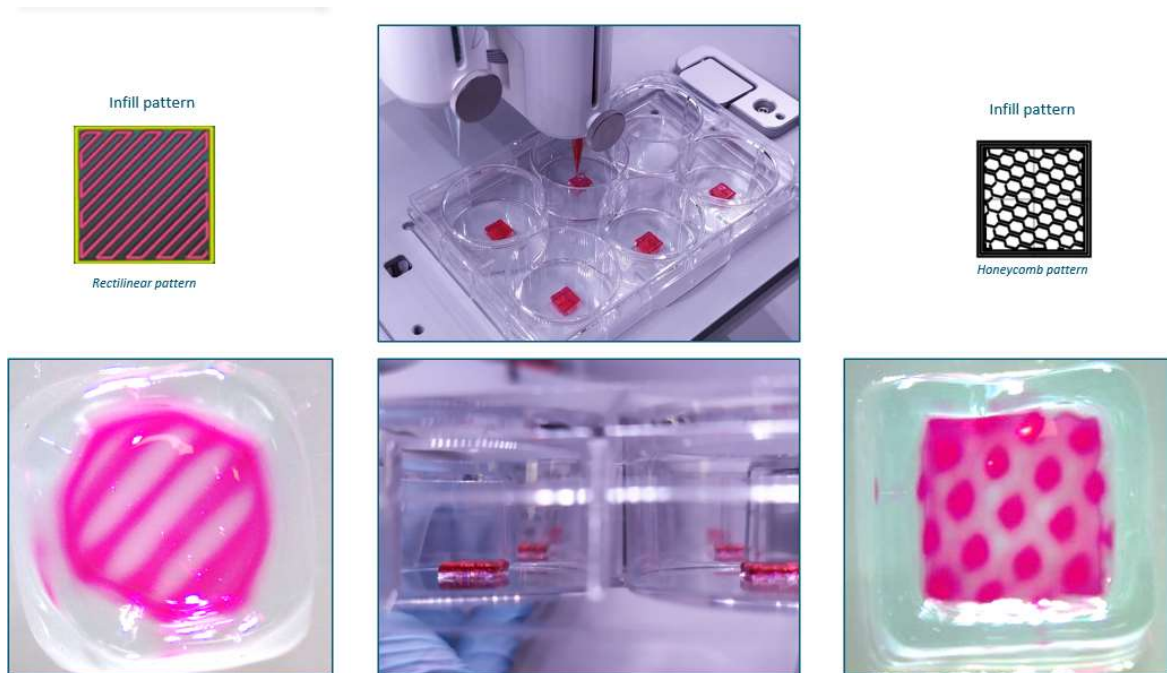
Figure 2. , 3D Printing designs with demonstration models to improve dermal-epidermal junction shape with rectilinear infill pattern (left) and Honeycomb infill pattern (right)
