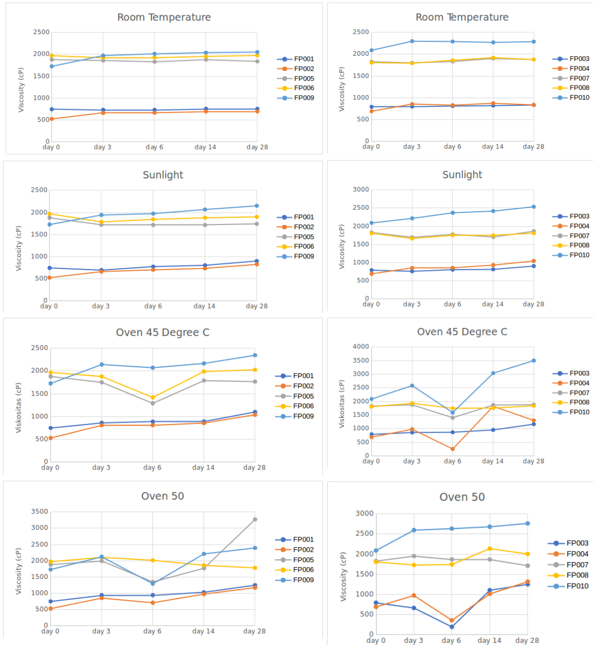
Figure 6. Graph of changes in viscosity with variations in the formulations of castor oil (left) and olive oil (right).
