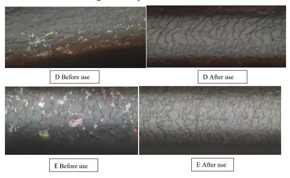
The result of experiment 3, through the test, the effect of D via the finger comb is the best. A, C, and D are comparable in toughness, and B and E are close to untreated.
