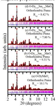
**Figure 1**: Observed (red filled circle), calculated (black continuous line) and difference profiles (blue continuous line) obtained after LeBail refinements of the synchrotron X-ray diffraction data of  $Dy_{(1-x)}Sm_{(x)}MnO_3$ . Vertical tick marks the Bragg peak positions.
