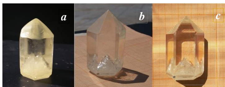
Figure 1. Single crystals of a) pure \alpha -LiIO 3 , b) \alpha -LiIO 3 doped with L-arginine and c) \alpha -LiIO 3 doped with L-nitroarginine.
