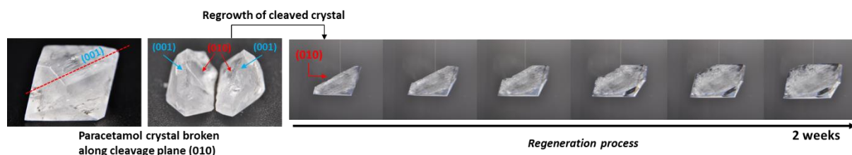
Figure 1. Regeneration process observed in a macroscopic paracetamol crystal broken along the cleavage plane (010)
