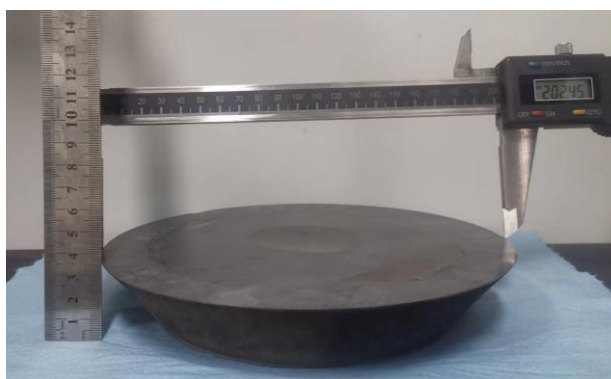
Fig. 1. Optical photos of 8-inch SiC ingot with a thickness of 40 mm
