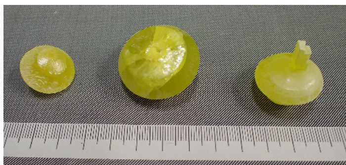
Fig. 1. Single crystals of OCCC grown Ce:GAGG.
