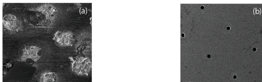
Figure 1. (a), SEM image shows barium sulfate precipitated in absence of ionophore and (b), SEM shows no precipitation in presence of calcium ionophore based on C. Figure based on [1]
